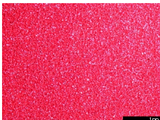
Microscopic view of the lack of blistering of the Atlas cell panel of Teflon ® 532-13054 system
