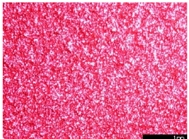
Microscopic view of the lack of blistering of the Atlas cell panel of Teflon ® 858-916 system
